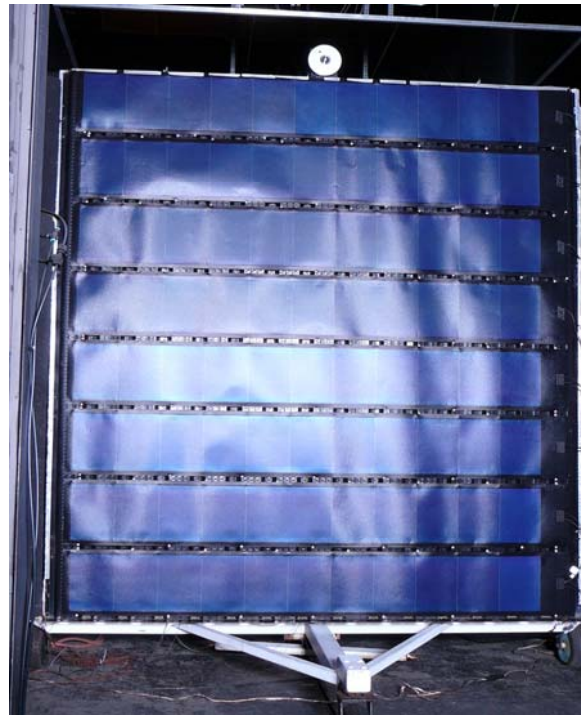
Fig. 5 PV/T testing with eight UniSolar 68 Watt modules
