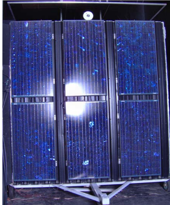
Fig. 4 PV/T testing with six BP 160 Watt panels
