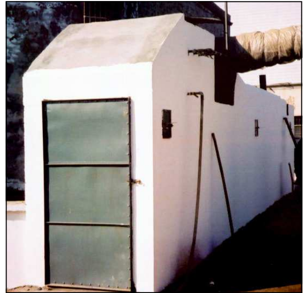
Tunnel dryer for jujube fruit
